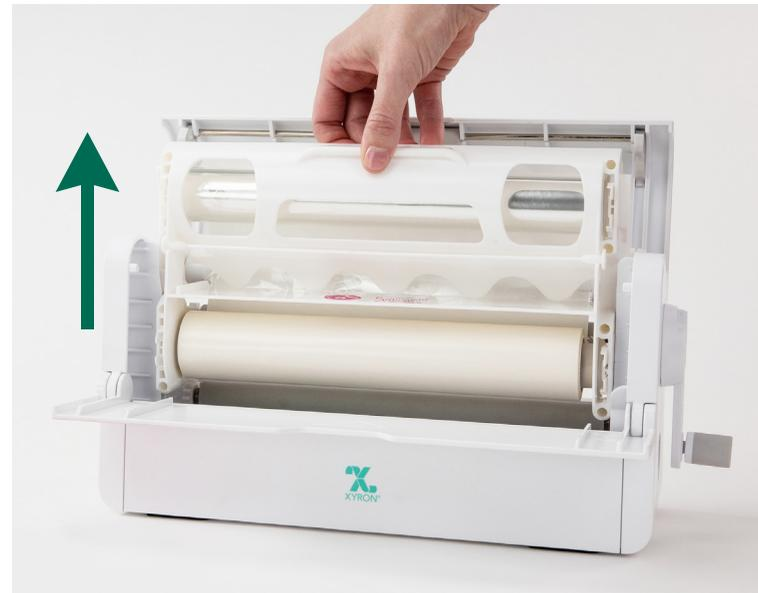
**2** Pull cartridge up and out of the machine.
