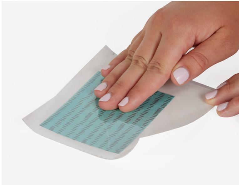
**1** After trimming from machine, rub item to ensure full adhesive transfer.
